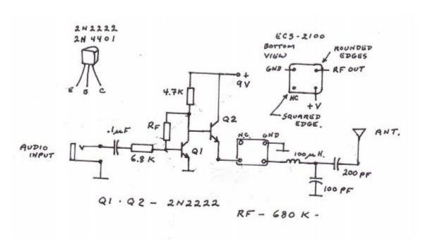
Audio may be from a CD player, an I-pad or microphone. Transistor Q1 provides voltage gain and transistor Q2 is the modulator.
