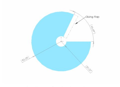
Figure 1 Flattened Cone Dimensions (radius shown)
