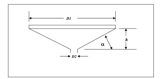
Measure the major diameter D1, the minor diameter D2 and the height h of the old cone.
