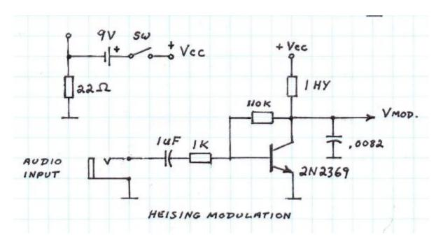
This QRP (low powered) broadcast transmitter was designed and built by Reed, W2CQH, to use at the SARS monthly meetings for those who brought in broadcast radios and wanted to show off how well they worked. The building where we meet is steel framed so reception is marginal at best, plus we can play our own selections of favorite music. I will say the fidelity is very good for such a simple device and the Heising modulation works quit well and seems to boost the effective power of the device.
